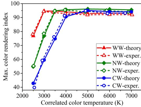
**Fig. 6** Experimental (dashed curves) and theoretical (solid curves) dependence of the maximal CRI from CCT for the three studied SLS.
