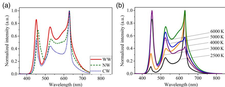
**Fig. 7** Examples of the spectra of the RGBW cluster with (a) WW, NW, and CW basic LED at 4000 K and (b) WW LED at different color temperatures.
