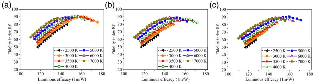
**Fig. 4** IES fidelity index Rf versus luminous efficacy for the CCT range of 2500 to 7000 K for RGBW systems with (a) basic warm, (b) neutral, and (c) cold white LED.
