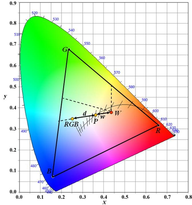
**Fig. 1** CIE  $x, y$  chromaticity diagram with schematic chromaticity coordinates of white, blue, green, and red LEDs ( $W, B, G,$  and  $R$ ), the point on the Planckian locus ( $P$ ), and resulting light of the colored LEDs ( $RGB$ ).
