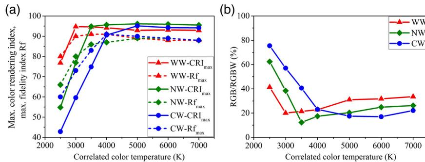
**Fig. 5** Maximal CRI (solid curves) and maximal fidelity index Rf (dashed curves) for the CCT range of 2500 to 7000 K for three RGBW systems with (a) different basic white LEDs and (b) the contribution of the RGB component to the resulting white light at these CRI<sub>max</sub>.
