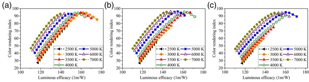
**Fig. 3** CIE CRI versus luminous efficacy for the CCT range of 2500 to 7000 K for the RGBW systems with (a) basic warm, (b) neutral, and (c) cold white LED.
