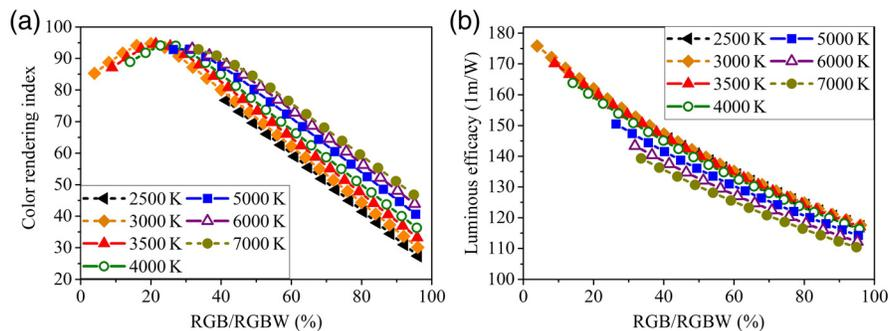
**Fig. 2** (a) CRI and (b) luminous efficacy versus RGB contribution for the CCT range of 2500 to 7000 K for the RGBW system with basic WW LED.
