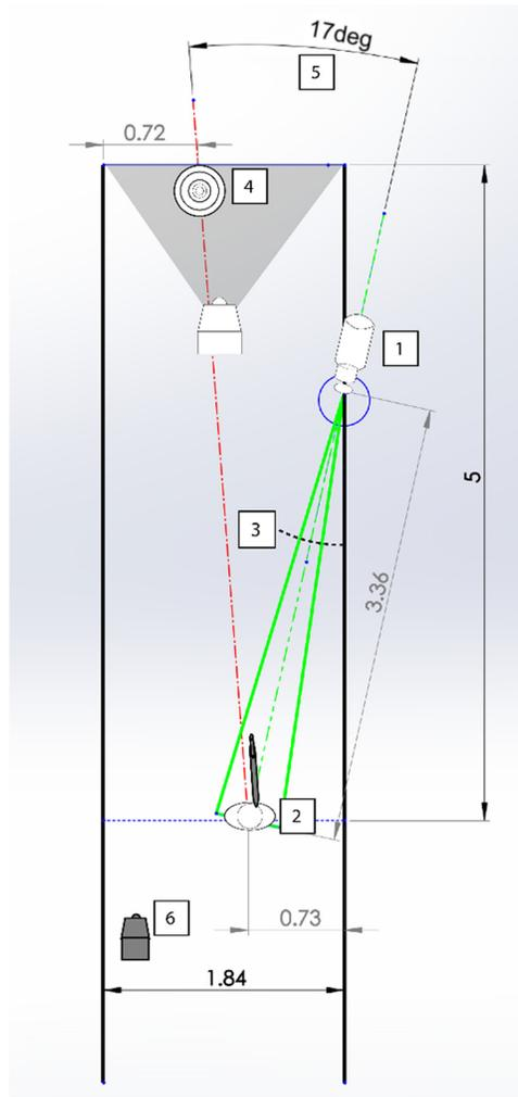
**Fig. 1** Scheme of the shooting simulator: 1, dazling laser; 2, shooter with modified gun; 3, beam from dazling laser; 4, projected target; 5, dazling angle; and 6, camera tracking the infrared spot of the weapon.
