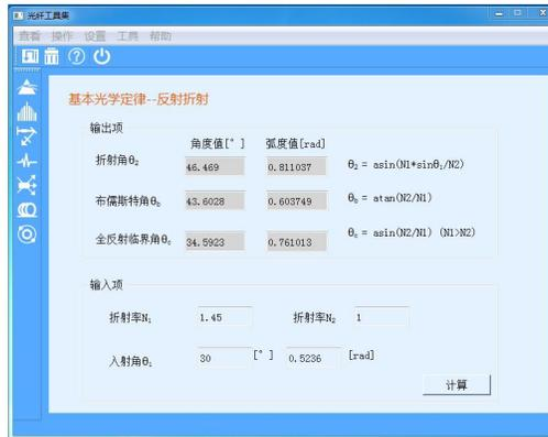
Fig. 2 Simulations on refracted angle and critical angle of the total reflection.
