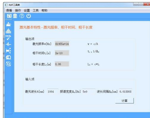
Fig. 3 Simulations on laser frequency, coherent time and length.
