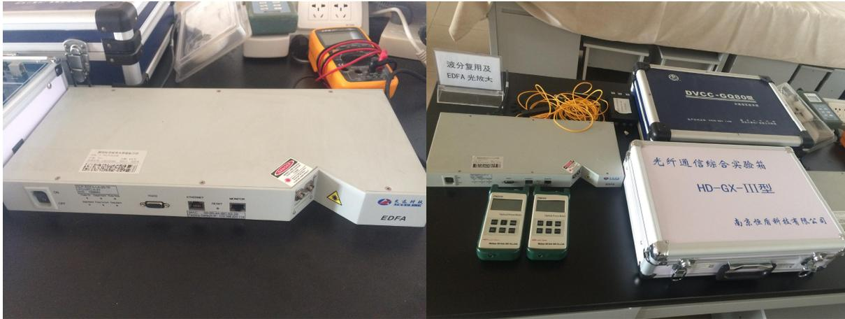
Fig. 11 Experimental setup on EDFA, WDM and fiber passive components.
