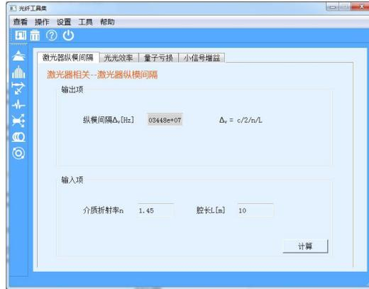
Fig. 4 Simulation on longitudinal mode spacing.
