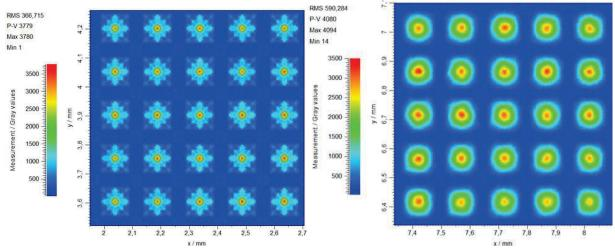
Figure 5: Spot image measured on Optocraft's Shack-Hartmann sensor UHR3 at a wavelength of 1064 nm. The array's lens pitch is 0.15 mm and the focal length is f = 13 mm (left) and f = 9.5 mm (right).
