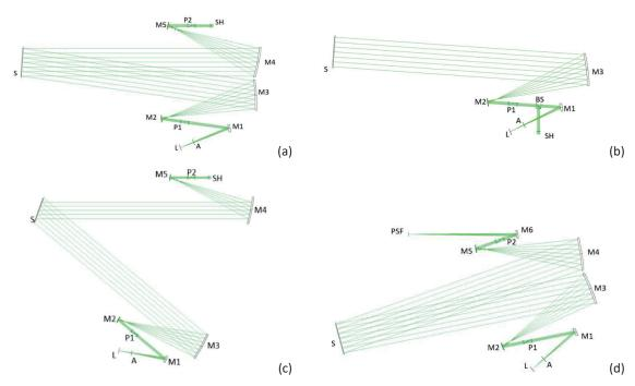
Figure 1: Optical setup of the bench for the wavefront measurement at 4° AOI (a), 0° AOI (b), at 20° AOI (c) and for the PSF measurement at 20° AOI (d).
