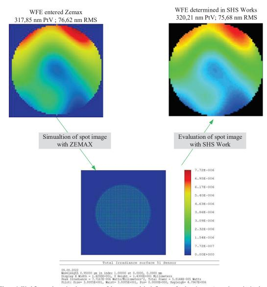
Figure 6: Workflow to determine the accuracy of the sensor and the influence of a ghost image. A spot image is simulated in ZEMAX with an incoming wavefront error. The SHS Works software is used to reconstruct the wavefront, including the ghost, from the simulated spot image.
