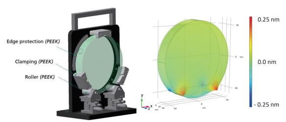
Figure 3: Specimen holder with positioning platform (left), simulated surface deformation in the Z direction (right).
