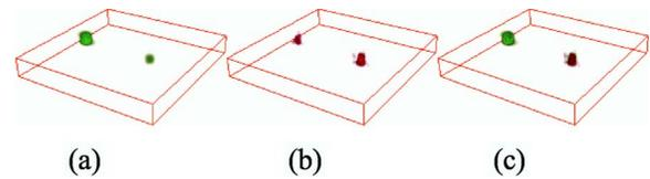
**Fig. 2** Three-dimensional reconstruction of MPM/OCT images of  $1\text{-}\mu\text{m}$ -diameter fluorescent beads. (a) TPEF image; (b) OCT image; (c) merged image. The image dimension is  $20 \times 20 \times 2.5 \mu\text{m}$ .
