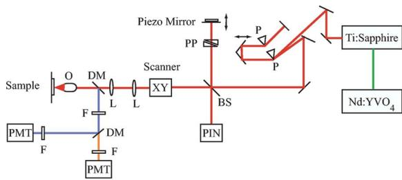
**Fig. 1** Schematics of the combined multiphoton and optical coherence microscopy system. BS: beam splitter; DM: dichroic mirror; F: filter; L: lens; O: objective; P: prism; PP: prism pair; PMT: photomultiplier tube.
