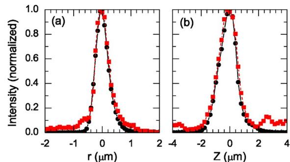
**Fig. 3** Transverse (a) and axial (b) point spread functions of MPM and OCT. The circles are for MPM and the squares are for OCT.
