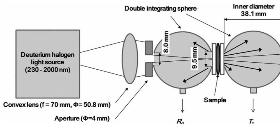
Fig. 1 Schematic of double integrating sphere setup.
