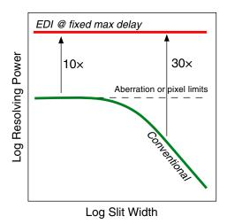
**Fig. 46** Notional diagram: the EDI surmounts classical limits to resolution from native spectrograph lens aberrations or detector pixel Nyquist sampling requirements. EDI resolution Res  $\sim \tau_{\text{max}}/\lambda$  is independent of slit width.
