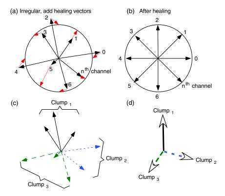
**Fig. 13** Regularizing an irregular phase set of fringing data (a) into a regular set (b) involves, for each input vector, adding small amounts of other data from the same set. In the presence of noise, it is beneficial to add averages (d), "clumps," of those data (c) facing similar directions.
