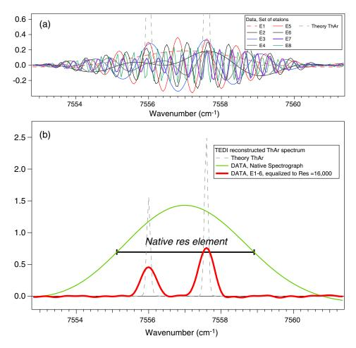
**Fig. 5** (a) Reconstruction of an otherwise unresolved ThAr doublet (7556, 7557.6 cm<sup>-1</sup>) from many wavelets measured at multiple delays. (b) The native spectrograph (green curve) cannot resolve the doublet. The EDI reconstructed spectrum (red curve), which is sum of wavelets, then equalized to RES = 16,000, easily resolves the doublet.
