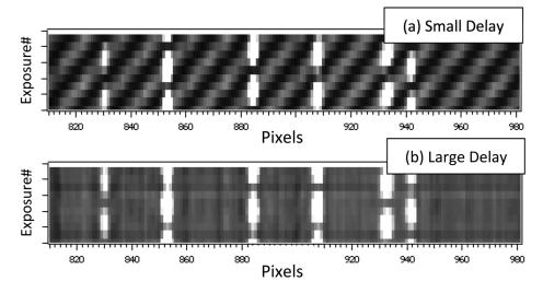
**Fig. 8** The 10 sequentially recorded phase stepped 1-D spectra are stacked versus exposure # (~phase) along the vertical. (a) Small delay (E1, 0.1 cm), the comb period is wide enough to be resolved. (b) Larger delay (E3, 0.7 cm), the comb is unresolved. ThAr phase pattern constitutes a "fingerprint" that reveals the precise interferometer delay. Un-normalized intensity fluctuations due to atmospheric seeing cause horizontal artifacts in (b). Horizontal scaling ~1 cm<sup>-1</sup> per pixel.
