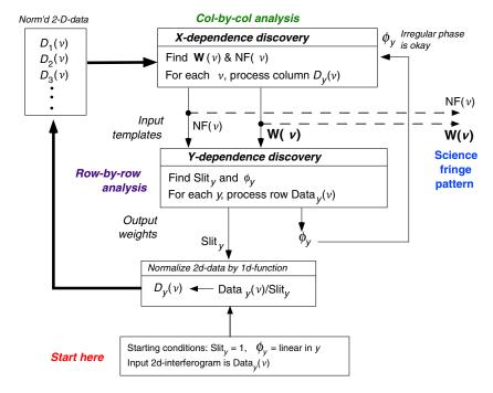
**Fig. 9** Flowchart of iterative strategy for finding phases and amplitudes of each row (phase step, Y) of the interferogram, while also finding the ordinary spectrum (nonfringing intensity NF) and the fringing spectrum value  $W(\nu)$  for each column (each X or  $\nu$ ). Slity is the phase (or channel) dependent intensity variations, due to atmospheric seeing, which we normalize out.
