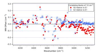
**Fig. 37** Irregular PSF drift of native spectrograph, versus wavenumber, correlated in 10 cm<sup>-1</sup> chunks between E6 and E1 (red dots), and E2 and E1 (blue open squares), for the A-order and September 19, 2010, data of HD219134. The time-dependent bulk offset (Fig. 36) has already been removed.
