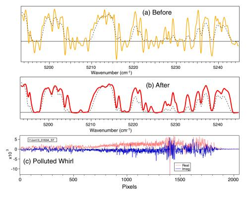
**Fig. 14** (a) Earlier spectral reconstruction results had excessive ringing (yellow curve), compared to telluric theory<sup>19</sup> (dashed). Bad normalization polluted the fringing signal (whirl) with nonfringing component, which created a pedestal-like offset in the whirl (c), which became ringing during heterodyning reversal frequency shift. (b) Ringing problem was solved (red curve) using a different normalization method.
