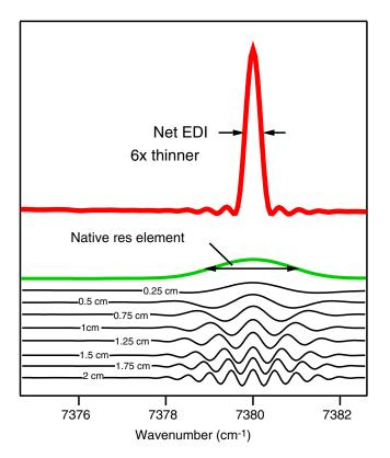
**Fig. 4** Simulated summation of several simulated wavelets, weighted in Gaussian equalization scheme, produces a single Gaussian PSF peak with minimal ringing (bold red) and thinner than the native spectrograph (green curve) by factors of several.
