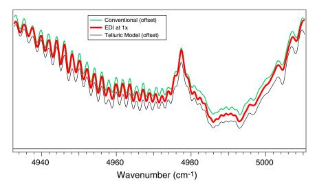
**Fig. 20** The EDI result (red, 1×) can provide an accurate measurement of the low-resolution information usually provided by the native spectrograph (green). Here we deliberately blur the fringing EDI result to the same resolution as native spectrograph. It accurately follows the details of telluric model (black). Green and black curves offset vertically. Target is star HD219134 + ThAr lamp, September 19, 2010.
