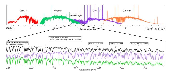
**Fig. 23** The TEDI reconstructed resolution boosted spectrum spans the four orders of TripleSpec spectrograph in NIR (4100 to 10,500 cm<sup>-1</sup>), here observing HD219134 on September 19, 2010. The lower graph is zoomed in region of overlapping orders B and C, showing agreement between two very unrelated groups of pixels (on opposite sides of detector), and with telluric model<sup>19</sup> (black curve).
