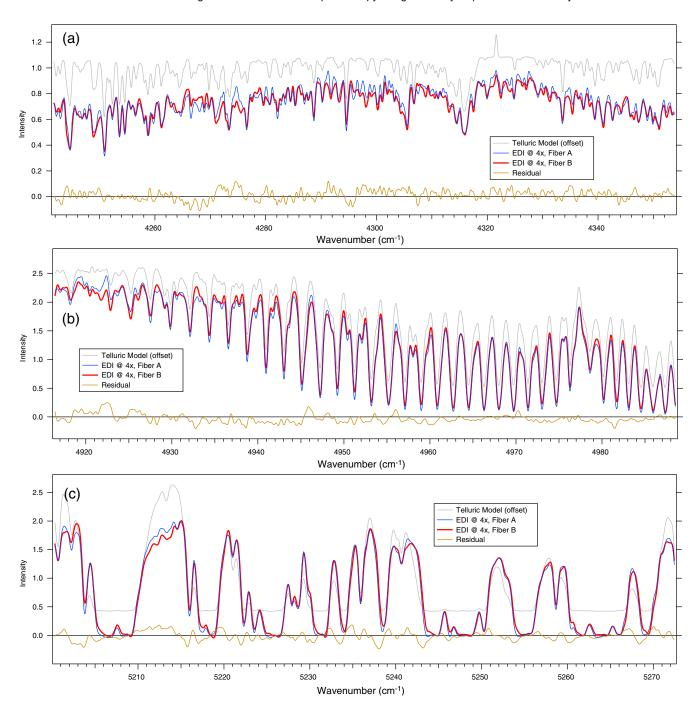
**Fig. 27** Additional regions of the A-order when comparing two fibers A (thin blue) and B (thick red) and their difference (tan); same data as Fig. 26. (a) 4240 to 4354 cm<sup>-1</sup>, (b) 4916 to 4989 cm<sup>-1</sup>, (c) 5200 to 5272 cm<sup>-1</sup>. Telluric model (gray) offset vertically.
