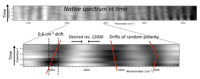
**Fig. 35** Large PSF irregularity in the native spectrograph to which EDI is robust. Row is native spectra of A-order versus etalon # ( $\sim$ 10 min apart). The PSF shift  $\sim$ 0.6 cm<sup>-1</sup> versus etalon # is called "shear." Bulk shear has already been removed here, and an irregularity remains. Note irregular change in shear polarity. Fortunately, for the EDI the native lineshape only affects the envelope of the wavelets, but not the internal shape.
