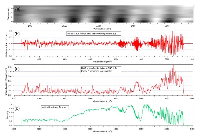
Fig. 38 (c) Measured amount of (vertical) instrumental noise for A-order, as a fraction of continuum, due to (horizontal) PSF drift or width change, by subtracting the native spectrum averaged over all eight etalons (d) from each spectrum (a) measured individually for each etalon to produce about a 3% residual (b).
