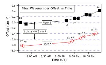
**Fig. 36** Bulk translation of the native spectrum along the dispersion axis due to thermomechanical or changing gravity vector, and due to slit slant acting on vertical separation of fibers A and B, for star HD219134 on September 19, 2010.
