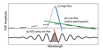
**Fig. 3** The EDI PSF (instrument response) is a corrugated peak (bold curve), which has a much higher slope (and thus higher Doppler sensitivity) than the low resolution native spectrograph alone (dashes). The slope of the sinusoid is proportional to the interferometer delay. For use in high-resolution spectroscopy, the subject of this report, the central area (cross-hatched) is made unambiguous by combining several wavelets of different periodicities (delays), as shown in Figs. 4 and 5.
