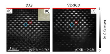
**Fig. 7** PAT imaging of printed dots array detected by single array. (a) Photograph of the phantom; (b) image reconstructed by DAS; and (c) image reconstructed by VR-SGD. The red line indicates the position of the transducer array. The ROIs for the signal and background are marked by the red and blue circles, respectively.
