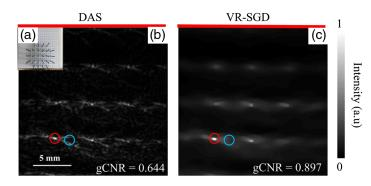
**Fig. 8** PAT imaging of pencil leads detected by single-array geometry: (a) photograph of the phantom; (b) image reconstructed by DAS; and (c) image reconstructed by VR-SGD. The red line indicates the position of the transducer array. The ROIs for the signal and background are marked by the red and blue circles, respectively.
