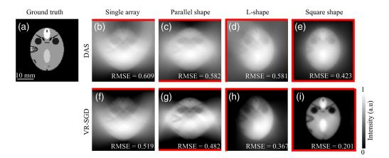
**Fig. 5** Reconstruction of the FORBILD phantom by single-array, parallel shape, L-shape, and square shape detection geometries, respectively. (a) Initial pressure distribution of the phantom; (b)–(e) reconstructed images by DAS; and (f)–(i) reconstructed images by VR-SGD after 30 iterations. Positioning of the linear arrays is indicated by the red lines. RMSE value is labeled in each reconstructed image.
