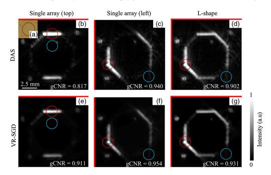
**Fig. 9** PAT images of octagon phantom detected by single-array and L-shape geometries. (a) Photograph of the phantom. (b)–(d) DAS reconstructed images by single array (top), single array (left), and L-shape detections, respectively. (e)–(g) VR-SGD reconstructed images for the corresponding detection geometries, respectively. Red lines indicate the orientation of the transducer array. The target and background ROIs are marked by the red and blue circles, respectively.
