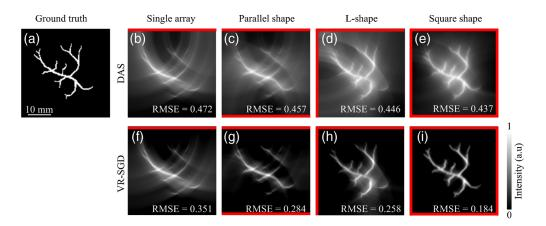
**Fig. 4** Reconstruction of the tree branch phantom by single-array, parallel shape, L-shape, and square shape detection geometries, respectively. (a) Initial pressure distribution of the phantom; (b)–(e) reconstructed images by DAS; and (f)–(i) reconstructed images by VR-SGD after 30 iterations. Positioning of the linear arrays is indicated by the red lines. RMSE value is labeled in each reconstructed image.
