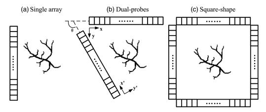
**Fig. 3** Detection geometries enabled by linear arrays: (a) single-array detection; (b) dual-probe geometry with an angle  $\theta$  (e.g., parallel-shape has  $\theta = 180$  deg and L-shape has  $\theta = 90$  deg); and (c) square-shape geometry with four probes.
