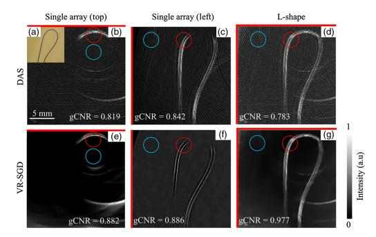
**Fig. 10** PAT images of a tube phantom detected by single-array and L-shape geometries. (a) Photograph of the phantom. (b)–(d) DAS reconstructed images by single array (top), single array (left), and L-shape detections, respectively. (e)–(g) VR-SGD reconstructed images for the corresponding detection geometries, respectively. Red lines indicate the orientation of the transducer array. The target and background ROIs are marked by the red and blue circles, respectively.
