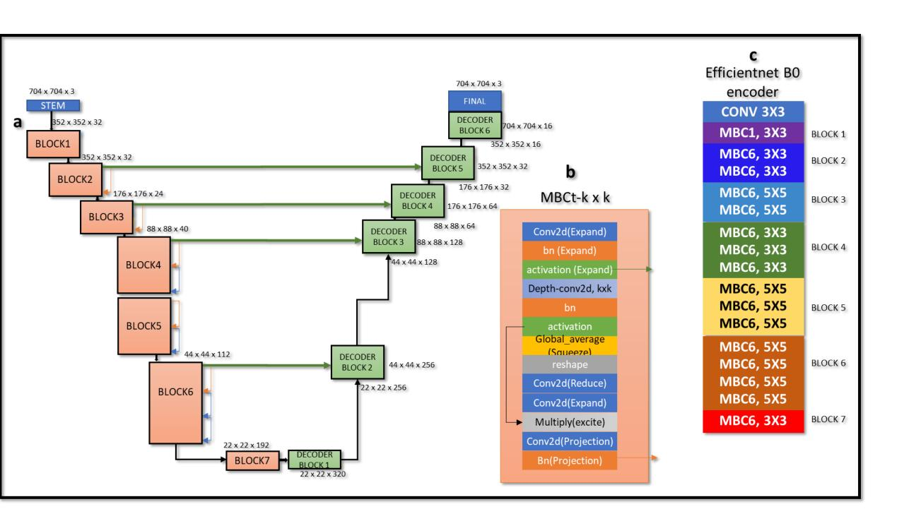
Fig. 3 Model architecture: Unet with efficientnetB0 encoder
